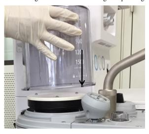
3. Hold the bellows housing tightly and turn it clockwise until it stops. Ensure that the side of the housing marked with scale is facing the operator.
