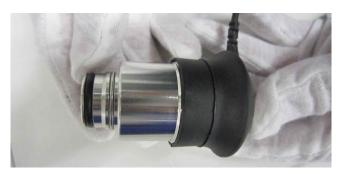
2. Insert the  $O_2$  sensor assembly into the  $O_2$  sensor port on the breathing system.
