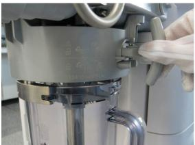
3. Pull out the CO<sub>2</sub> absorbent canister from the mounting slot.
