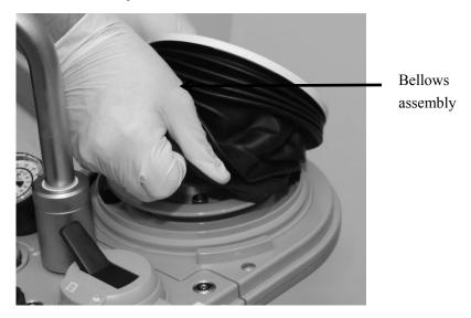
4. Remove the bellows top plate from the bellows assembly.
