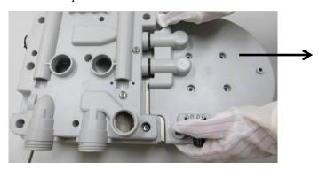
8. Erect the breathing system, and remove the six screws on the upper and lower panel of gauge base by inner hexagon spanner (5.0) and inner hexagon spanner (4.0).
