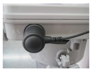
3. Unscrew the  $O_2$  sensor from the  $O_2$  sensor port on the breathing system.
