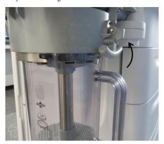
2. Turn the rotary handle for 90 degrees counterclockwise.
