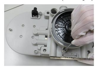
4. Lift off and remove the bellows base with the three screws.
