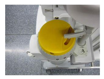
2. Rotate the self-locking device clockwise to fix the vaporizer onto the manifold.
