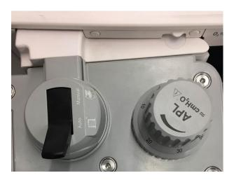
3. Lock the breathing system. Refer to *11.1.1.8 Install the CO2 Absorbent Canister* for operation steps. The process of installing the CO<sub>2</sub> absorbent canister is the process of locking the breathing system.
