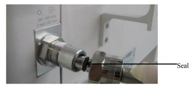
3. Ensure that the hode is properly connected and tighten the tube nut.
