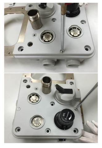
11. Remove the upper panel of gauges base.
