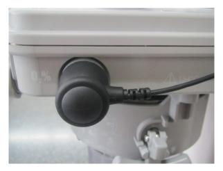
3. Insert the other end of the  $\mathrm{O}_2$  sensor cable into the  $\mathrm{O}_2$  sensor connector on the circuit adapter.
