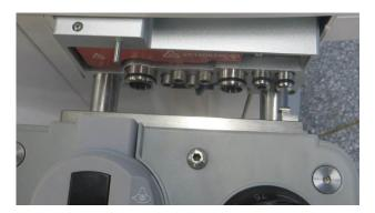
2. Push the breathing system into the circuit adapter firmly to allow the breathing system to be connected to the adapter seamlessly.
