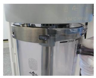
5. Turn the rotary handle clockwise for 90 degrees.
