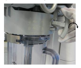
6. Let the rotary handle fall to lock the  $CO_2$  absorbent canister.
