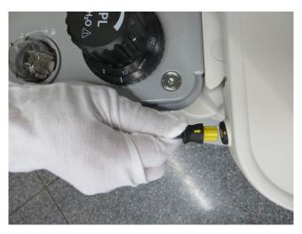
2. Remove the  $O_2$  sensor from the  $O_2$  sensor port on the breathing system.
