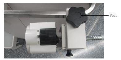
4. Insert the suction tube into the overfill protection connector. Then lift the nut and adjust the direction of the suction opening at the same time. Lower the nut after adjusting direction properly.
