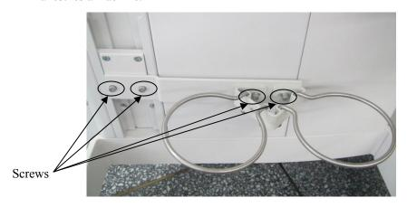
2. Place the liquid collection bottles into the rack. Install the suction tube based on the silkscreen on the liquid collection bottle.
