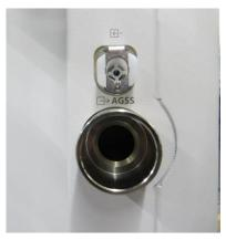
The outside diameter of the AGSS outlet is 30 mm. with 1:20 taper ratio. Please connect to the AGSS or waste gas disposal system.
