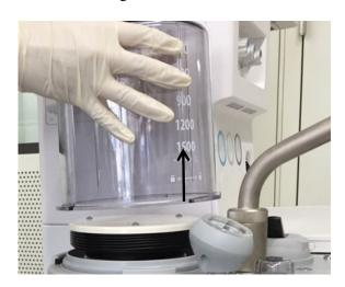
3. Remove the bellows assembly from the bellows base.
