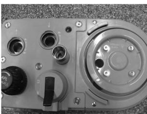
3. Unscrew the three screws of the bellows base by inner hexagon spanner (3.0).
