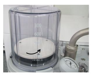
2. Lift off and remove the housing.
