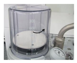
2. Lift off and remove the housing.
