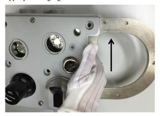
12. Separate the metal plate and the lower panel of gauge base.
