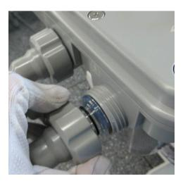
4. Tighten the locking nuts clockwise.
