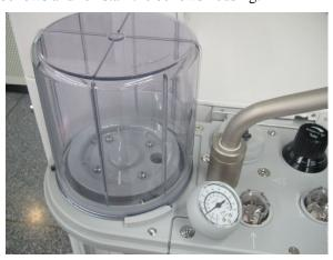
5. Plug the Y-piece of the breathing circuit into the leak test port to close the breathing system.
