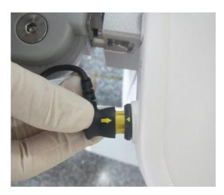
2. Remove the  $O_2$  sensor cable from the  $O_2$  sensor.
