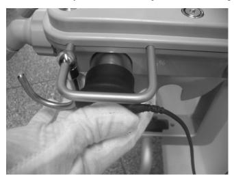
3. Insert the other end of the  $O_2$  sensor cable into the  $O_2$  sensor port on the circuit adapter.
