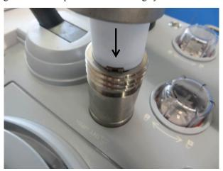
2. Turn the locking nut clockwise to tighten the bag arm.
