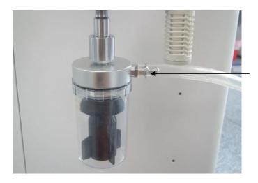
Insert the suction tube into the overfill protection connector
